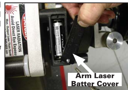
Figure 23 - Replacing Arm Laser Battery
