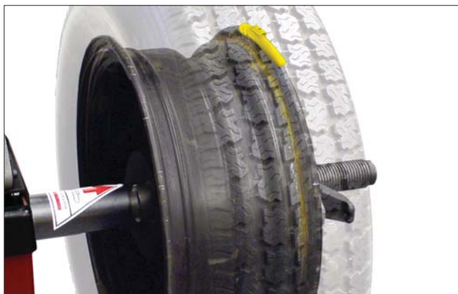
Figure 20 - Calibration Weight On Outside Flange At Top-Dead-Center
