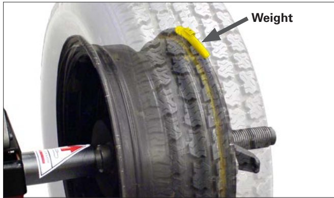
Figure 40 - Calibration Weight On Outside Flange At Top-Dead-Center
