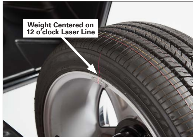
Figure 19 - Centering Corrective Weight At 12 o'clock Laser Line Location
