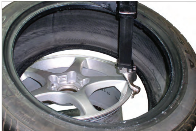
Figure 19 - Position Tire Against Mount/Demount Tool
