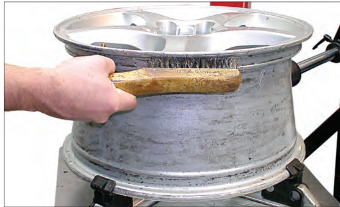
Figure 17 - Inspect and Clean the Wheel
