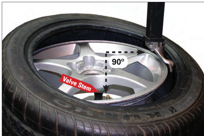
Figure 21 - Position Valve Stem 90° Ahead of Mount Tool
