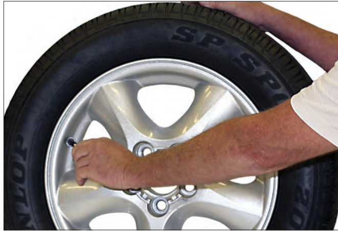
Figure 1 - Remove Valve Core to Deflate Tire
