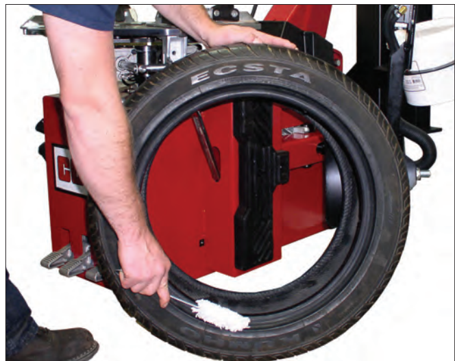
Figure 18 - Lubricate Tire Beads Liberally
