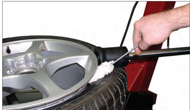
Figure 10 - Apply Rubber Lubricant to the Beads
