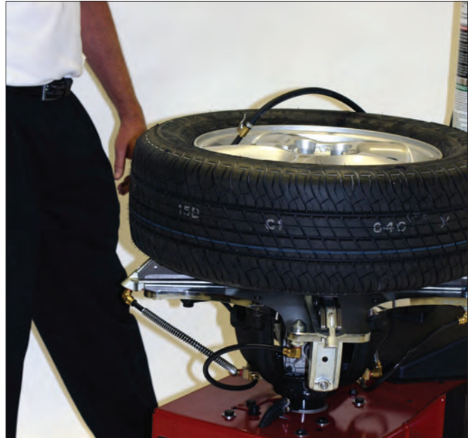
Figure 25 - Stand Back during Bead Seat
