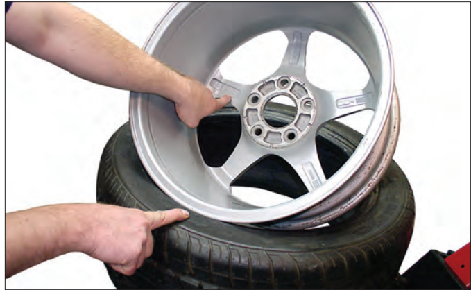
Figure 16 - Verify Size Match Between Tire and Wheel
