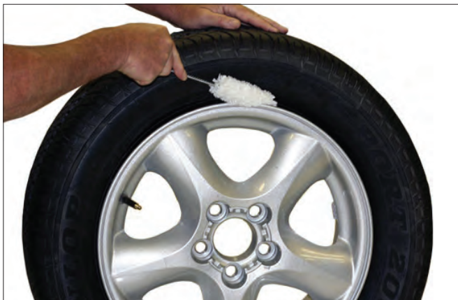
Figure 5 - Apply Rubber Lubricant to Tire Beads
