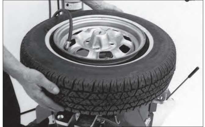
Figure 24 - Lift Tire Upwards for Bead Sealing
