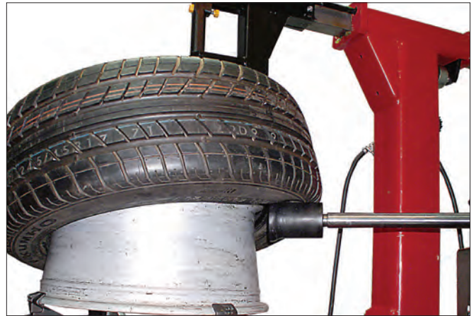
Figure 13 - Position Lower Horizontal Power Roller
