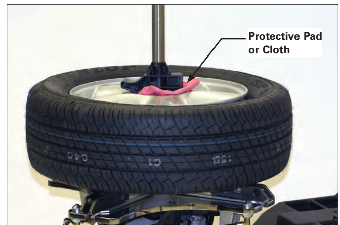
Figure 7 - Robo-Assist Aids Clamping
