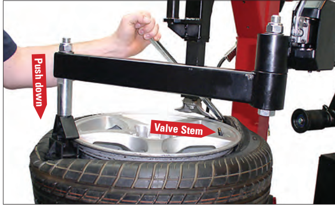
Figure 11 - Insert Bead Lifting Tool
