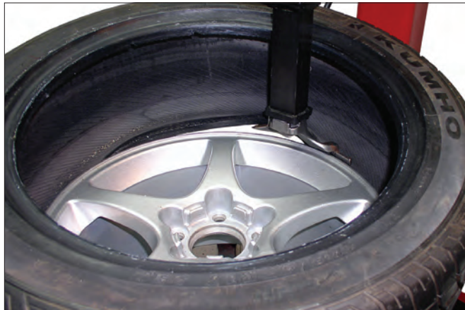
Figure 20 - Mounting Lower Bead
