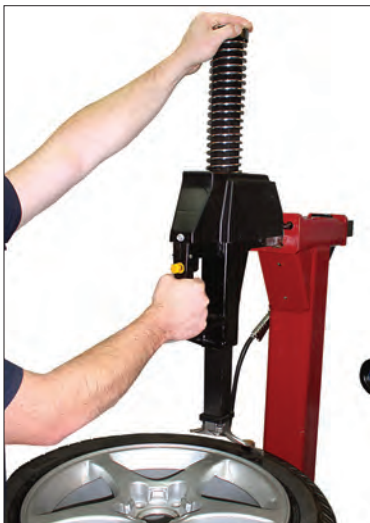
Figure 9 - Position Mount/Demount Tool
