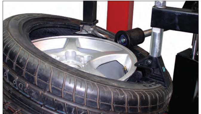
Fig 22 - Use Robo-Assist To Hold Tire In Rim Drop Center
