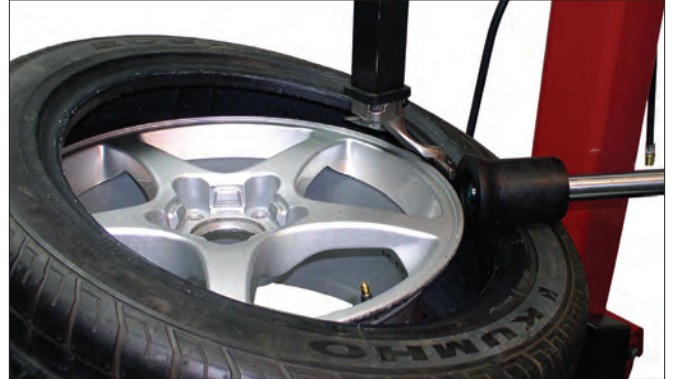
Fig 21a - Use Power Roller To Hold Tire In Rim Drop Center
