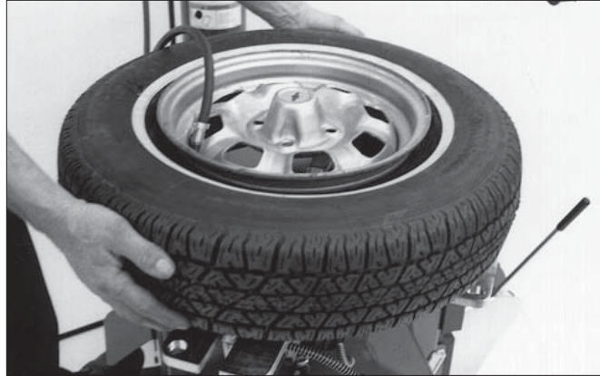
Figure 24 - Lift Tire Upwards for Bead Sealing
