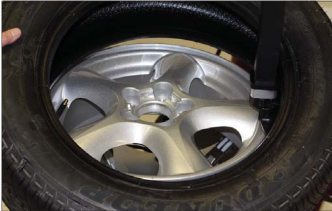
Figure 19 - Position Tire Against Mount/Demount Tool
