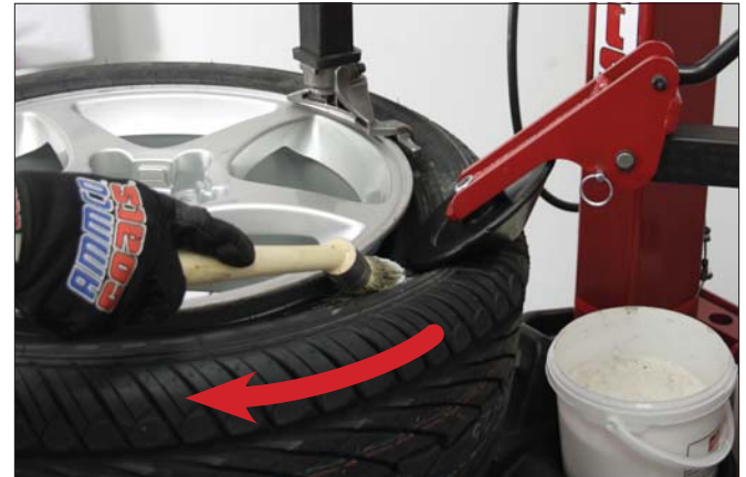
Figure 10 - Apply Rubber Lubricant to the Beads
