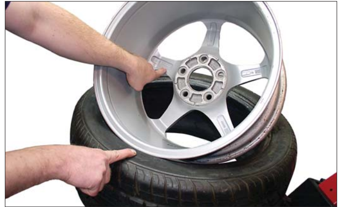
Figure 16 - Verify Size Match Between Tire and Wheel
