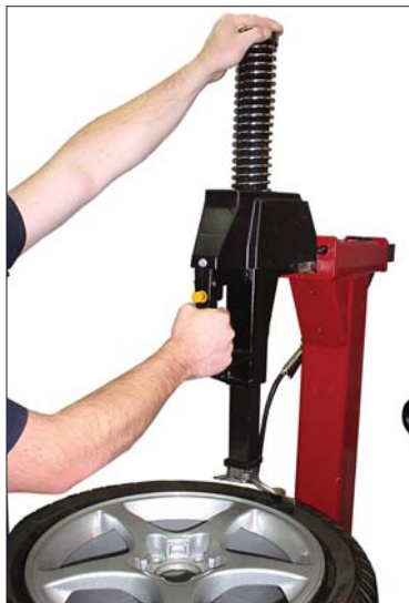
Figure 9 - Position Mount/Demount Tool
