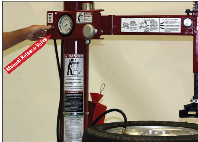
Figure 26 - Location of Manual Release Valve
