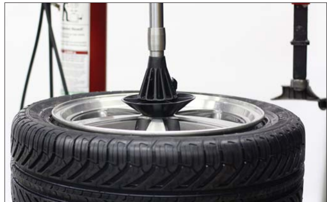
Figure 7 - Robo-Arm® Aids Clamping
