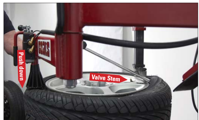
Figure 11 - Insert Bead Lifting Tool
