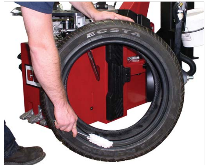
Figure 18 - Lubricate Tire Beads Liberally
