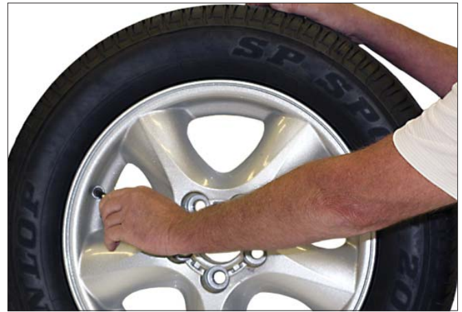
Figure 1 - Remove Valve Core to Deflate Tire
