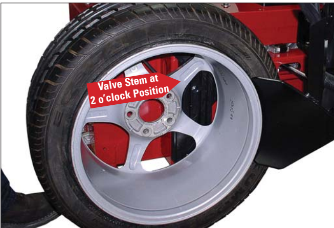
Figure 4 - Position Tire and Bead Loosener Shoe With Wheel Turned Around and Valve Stem in 2 o'clock Position.
