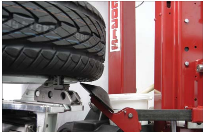
Figure 14 - Disk-assist Aiding Lower Bead Demount
