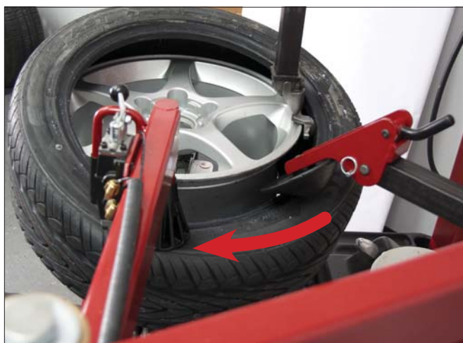
Fig 21 - Hold Tire Bead In Rim Drop Center
